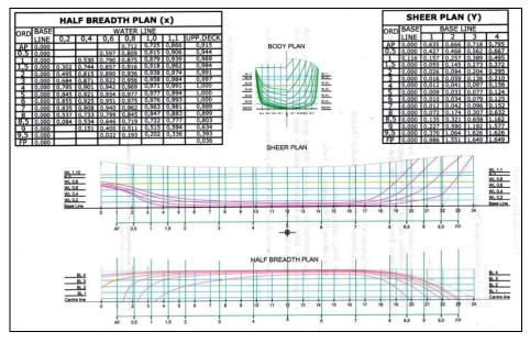
Figure 2: The Longline vessels lines plan
